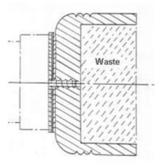
Attach the blank to a screw chuck and shape the outside as shown opposite. If you are going to drill the hole for the mechanism with a sawtooth drill cut a recess 1.5 inches in diameter as shown. This will make it easier to locate the drill in the centre of the piece. Not everyone will have a 1.5 inch drill so an alternative method of forming the hole will be described below in step 3. Sand and finish. Drill a pilot hole for the for the screw and reverse on the screw chuck ready for step two.
