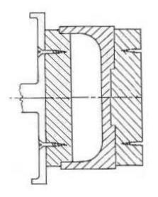
Mount another piece of scrap wood on the face plate and turn it away to accept the base as a snug fit. Now turn off the scrap wood attached to the base
